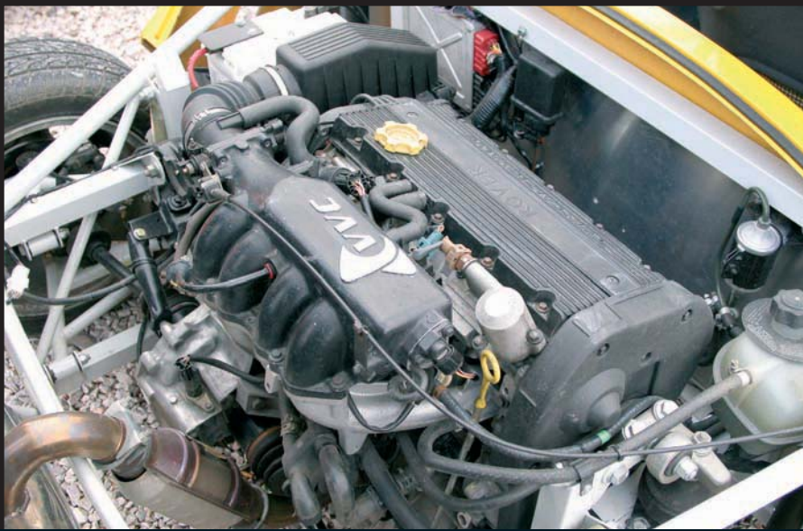
1.8-litre VVC engine in our 5EXi feels less urgent than non-VVC of orange car; Wood trim from Rover donor looks out of place.
